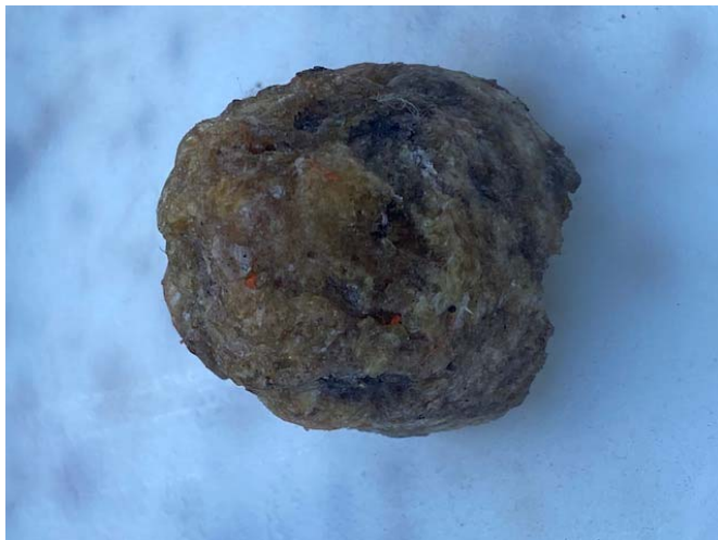
← This sample was obtained from approximately 11.5 feet below grade SPT B-3.
