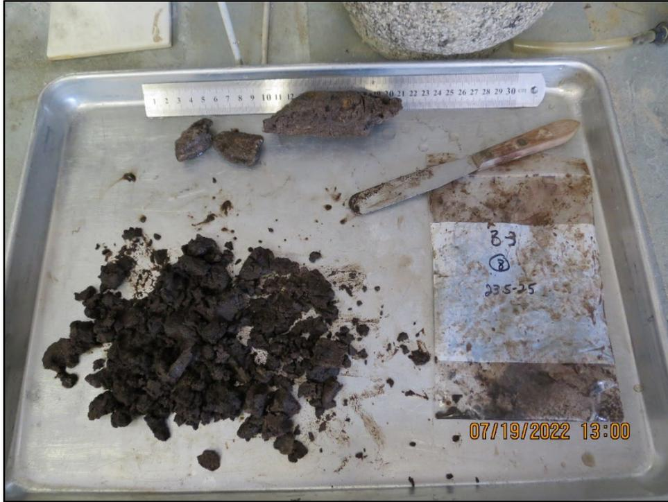
**Plate 1 – Polymer Retrieved in Split Spoon Boring B-3 from 23.5 to 25-feet below grade
