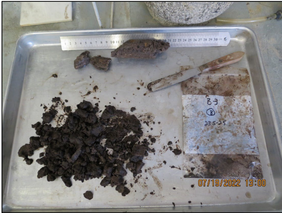
Plate 1 – Polymer Retrieved in Split Spoon Boring B-3 from 23.5 to 25-feet below grade (N=24 medium dense – previously WR)
