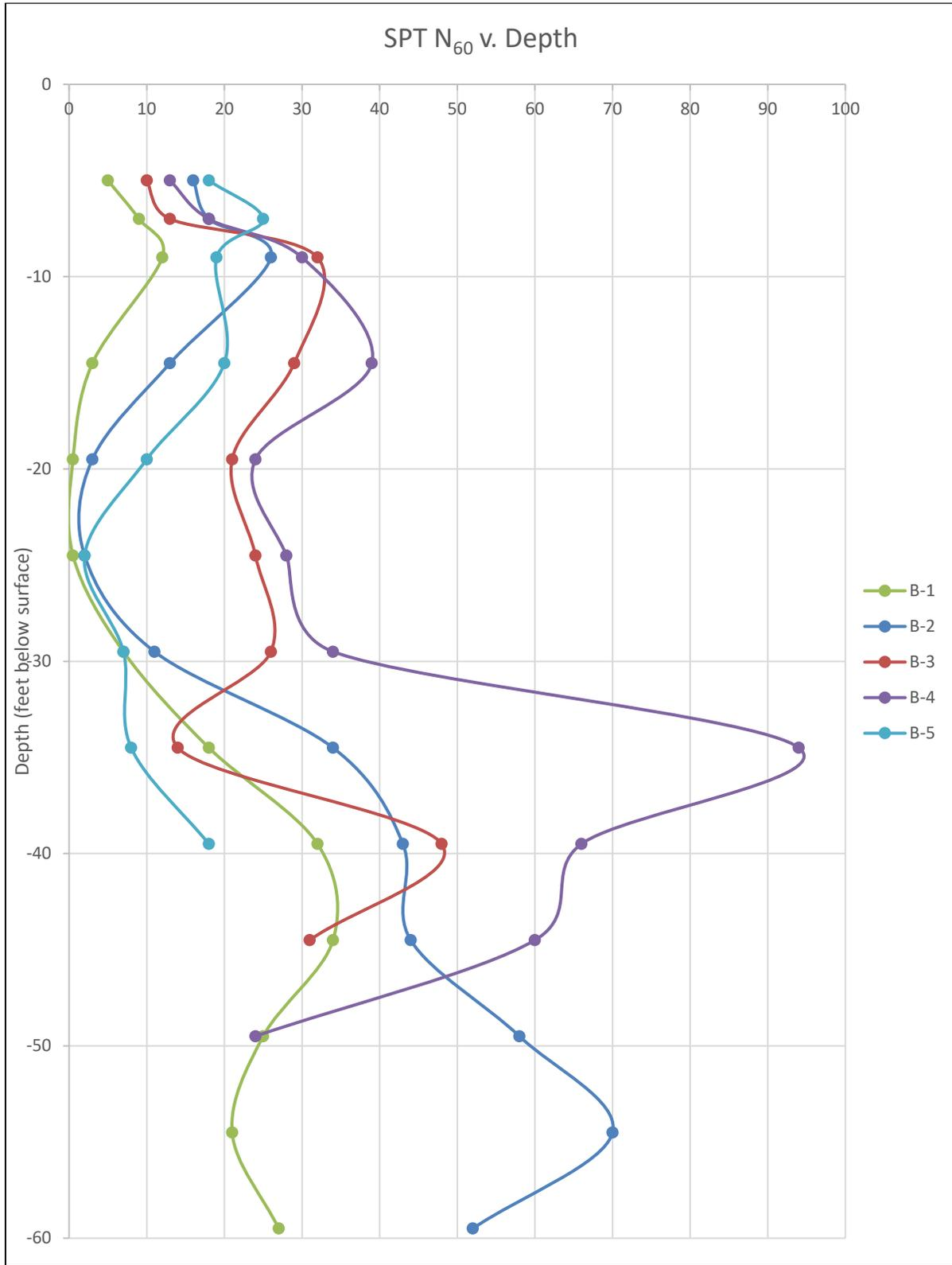
**Figure 1 – SPT N<sub>60</sub> vs. Depth (Pre- and Post-Treatment)**
