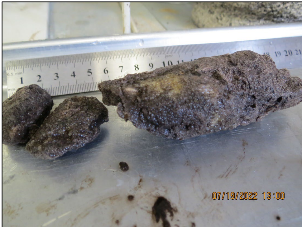
Plate 2 – Close up of Polymer retrieved from SPT at 25-feet
